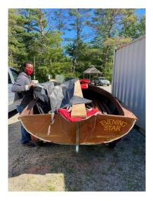
caulking back in it, and let it swell up, which is what I did when I got it, or one could replace the bottom plank with like kind, which is what I would do, or, one could glue and fasten 1/8 inch plywood over the bottom plank and add fiberglass over it. A good project for you all!
